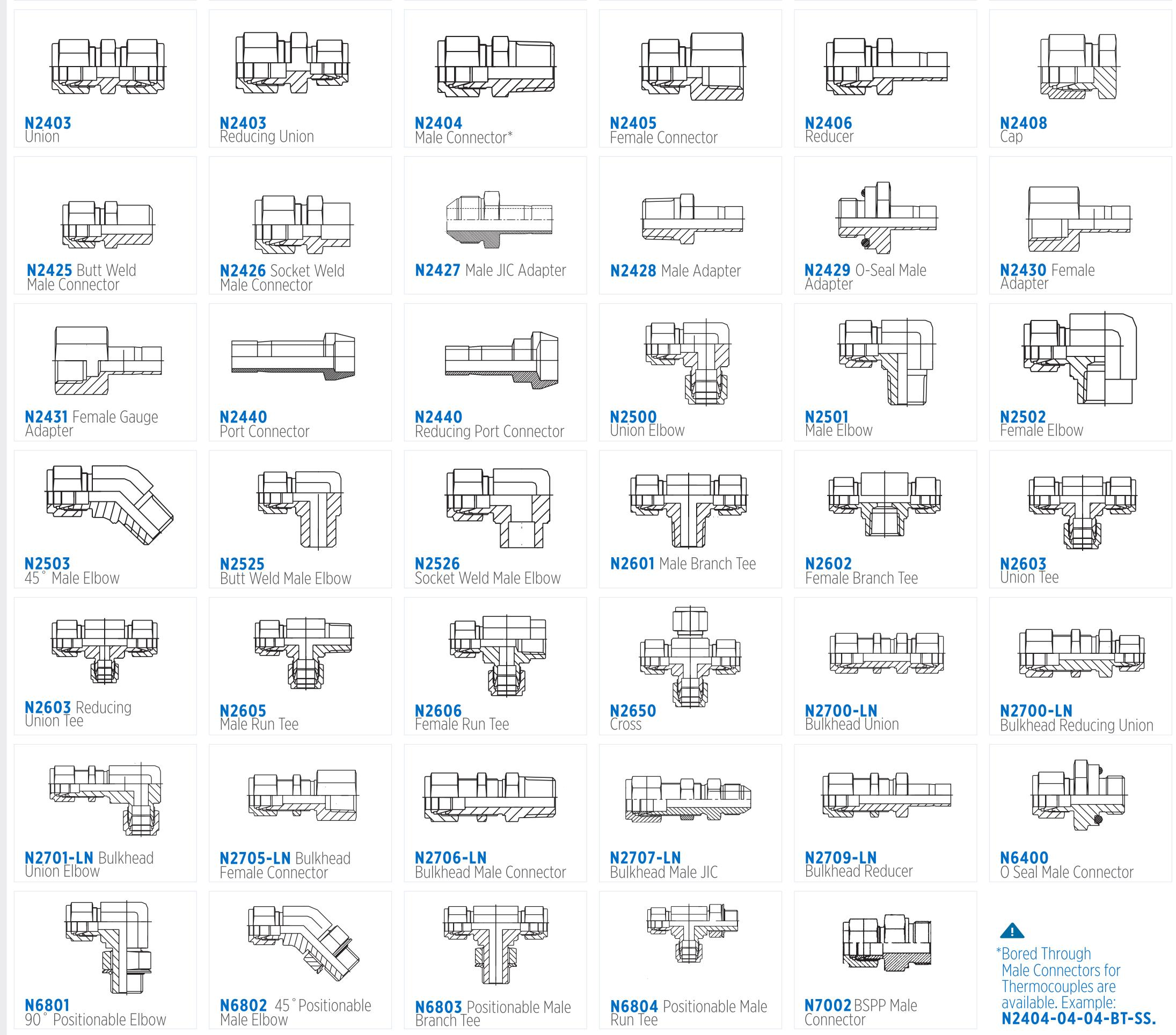
Brass and Stainless Steel available in Double Ferrule (N) and Single Ferrule (NS). Instrumentation valves available upon request.
